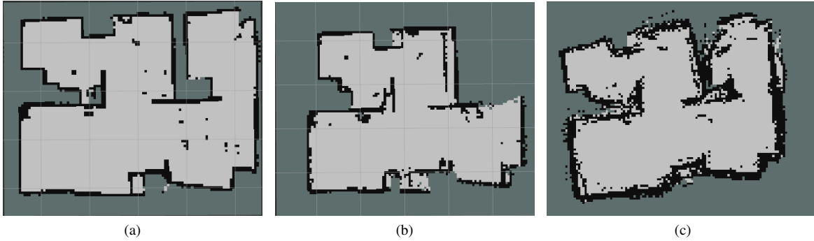
Fig. 5: Comparison of SLAM-generated maps: a) Baseline map generated using unmodified LiDAR measurements, b) Partially modified map during injection, c) Map during injection of corrupted LiDAR data.
